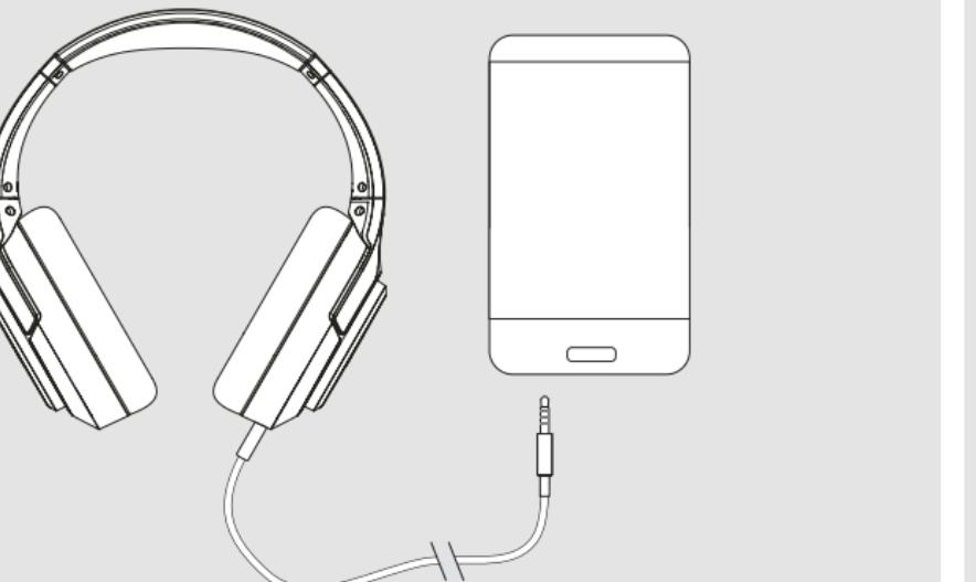
Connect the cable to the 3.5mm output on the mobile device.
